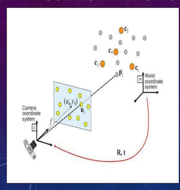
Pose estimation using the PnP algorithm involves calculating the 3D position and orientation of an object relative to a camera.
