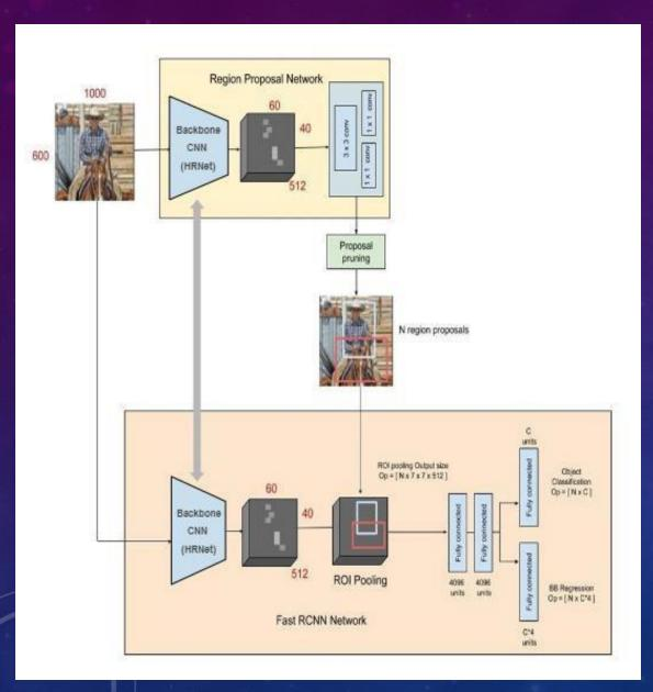
Faster R-CNN with an HRNet backbone is a powerful model for object detection, combining precise region proposal generation with detailed object classification and bounding box refinement.
